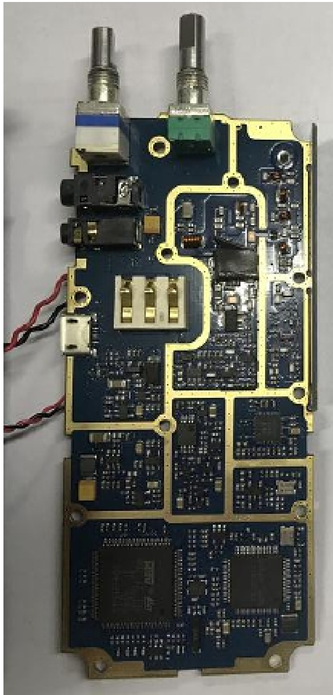
RF board without Shields (Bottom) (BC250D)
