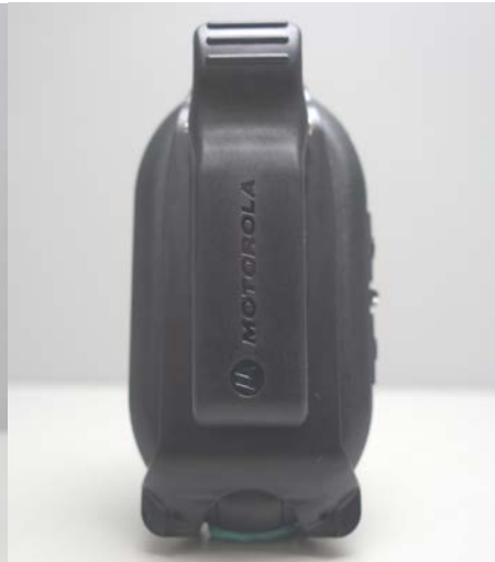
DUT Back View Swivel belt holster HKLN4438B
