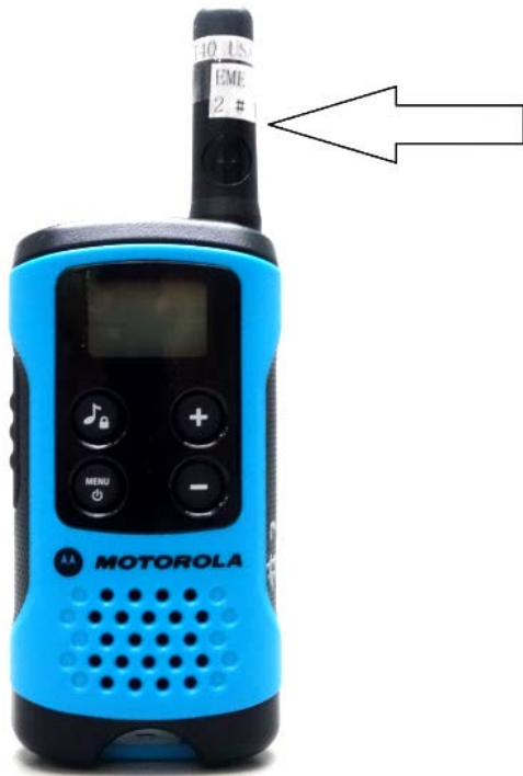
Fixed antenna pointed with arrow
