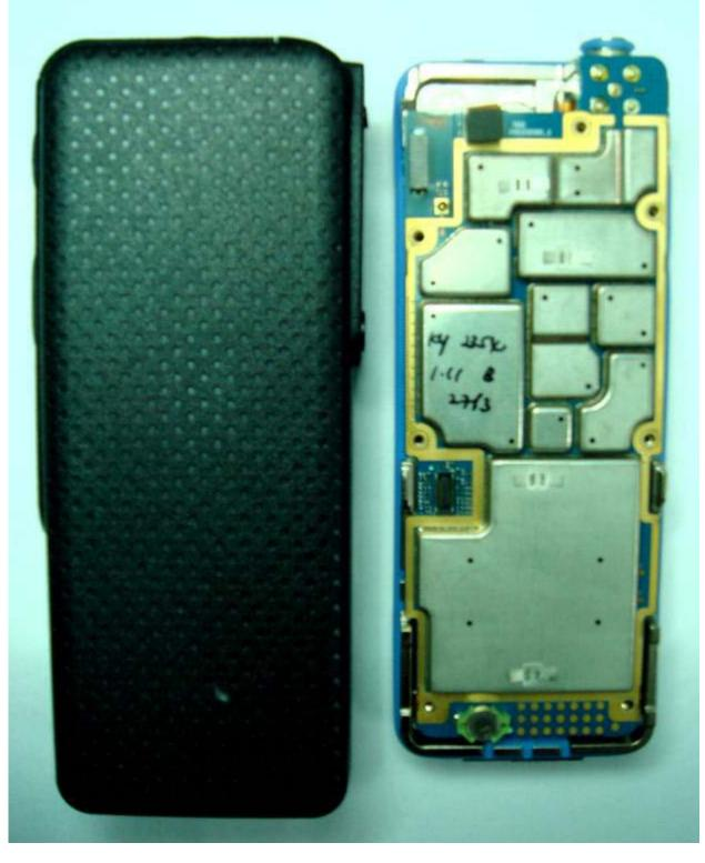
RF board with chasis and housing (front side)
