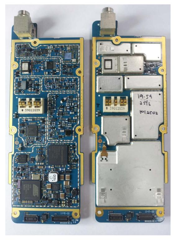
RF board without & with Shields (Bottom)
