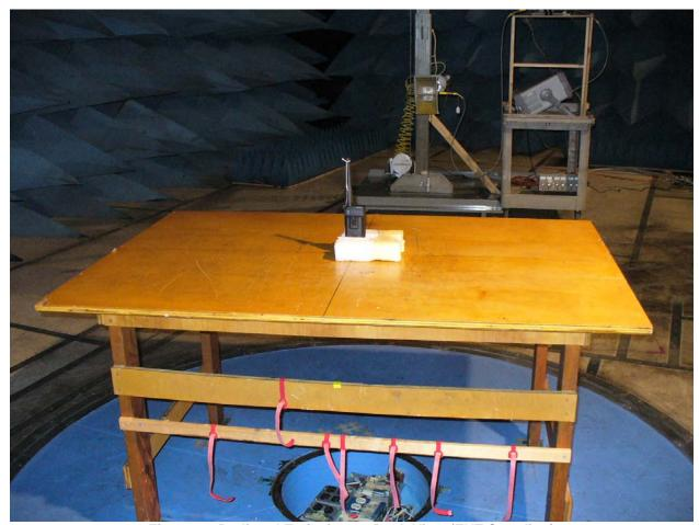
Figure 2: Radiated Emissions – Back View (EUT Standing)
