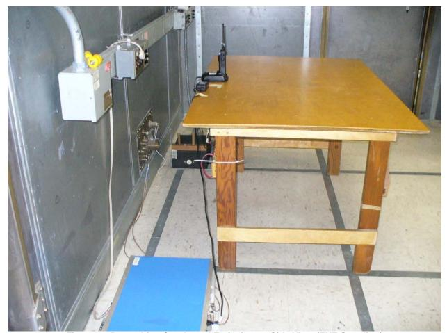
Figure 9: Power Line Conducted Emissions – Side View (EUT Standing)
