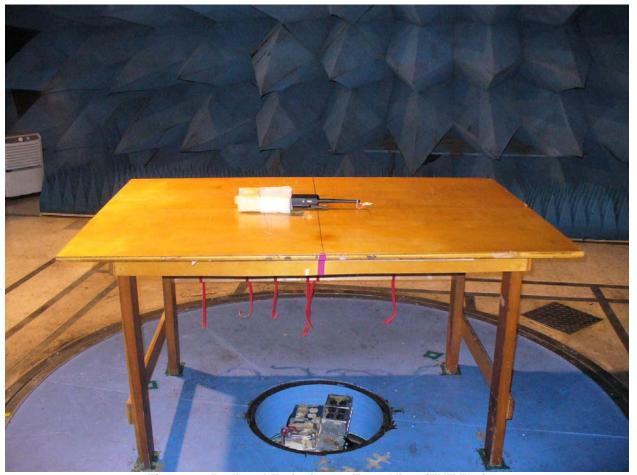
Figure 3: Radiated Emissions – Front View (EUT Flat)
