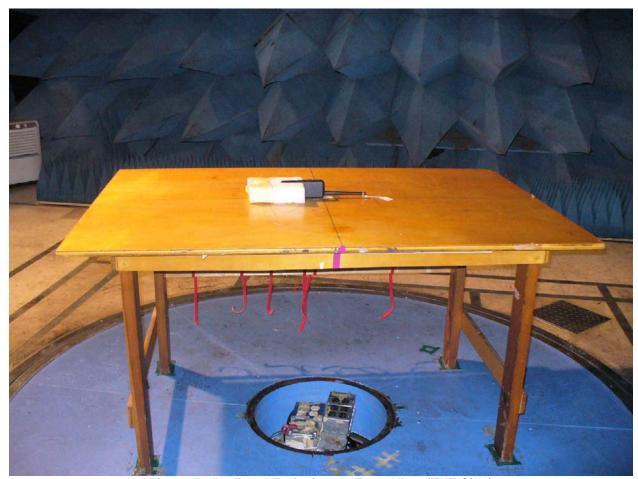
Figure 5: Radiated Emissions – Front View (EUT Side)
