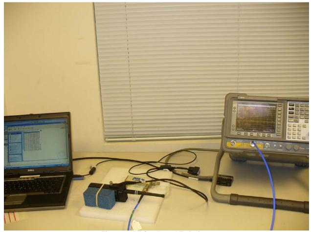
Figure 7: RF Conducted Emissions
