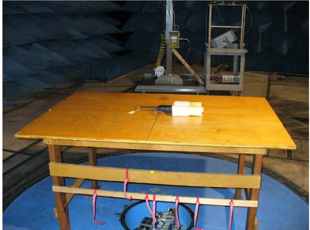
Figure 4: Radiated Emissions – Back View (EUT Flat)
