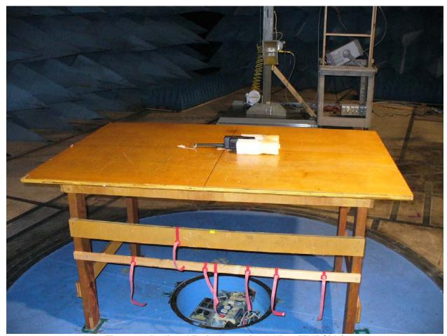
Figure 6: Radiated Emissions – Back View (EUT Side)
