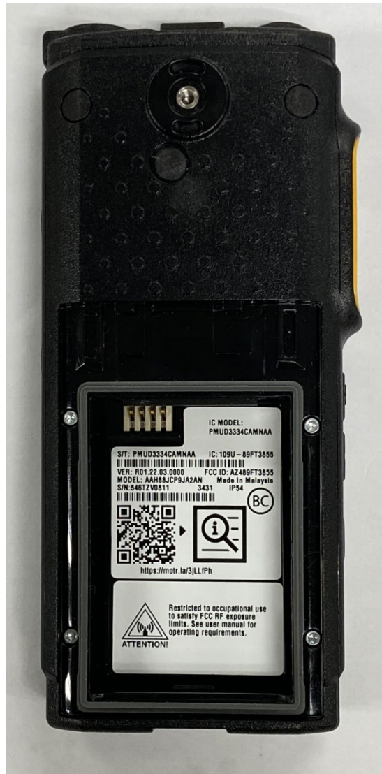
View of FCC/IC label location (SL300 - Display model)
