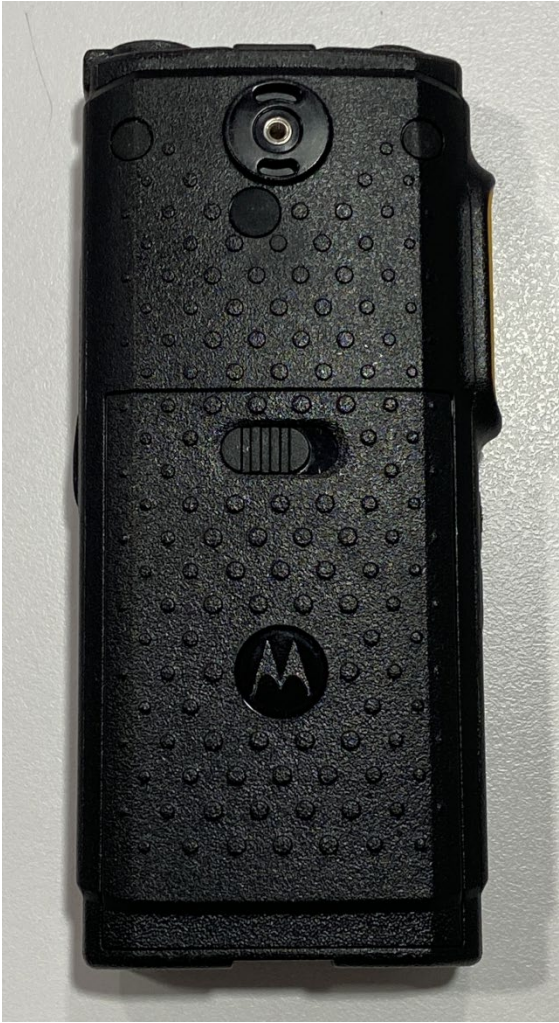
Back View with Battery & Battery Cover (SL300 - Display & Plain model)
