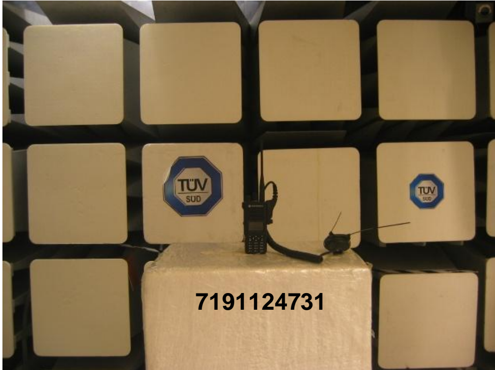
Transmitter Spurious Emissions (Radiated) Test Setup (Front View)
