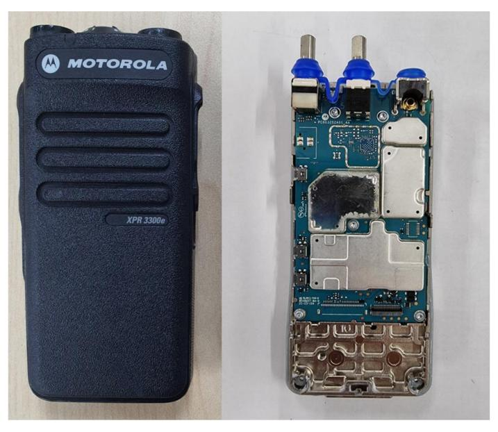
RF boards with chassis and housing for Non Keypad model (Front Side) TIA4950
