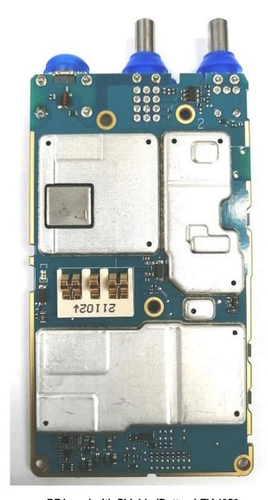
RF board with Shields (Bottom) TIA4950
