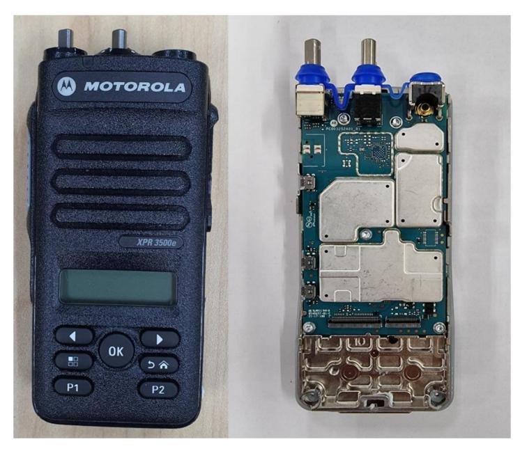
RF boards with chassis and housing for Display and Limited Keypad model (Front Side) Non-TIA4950
