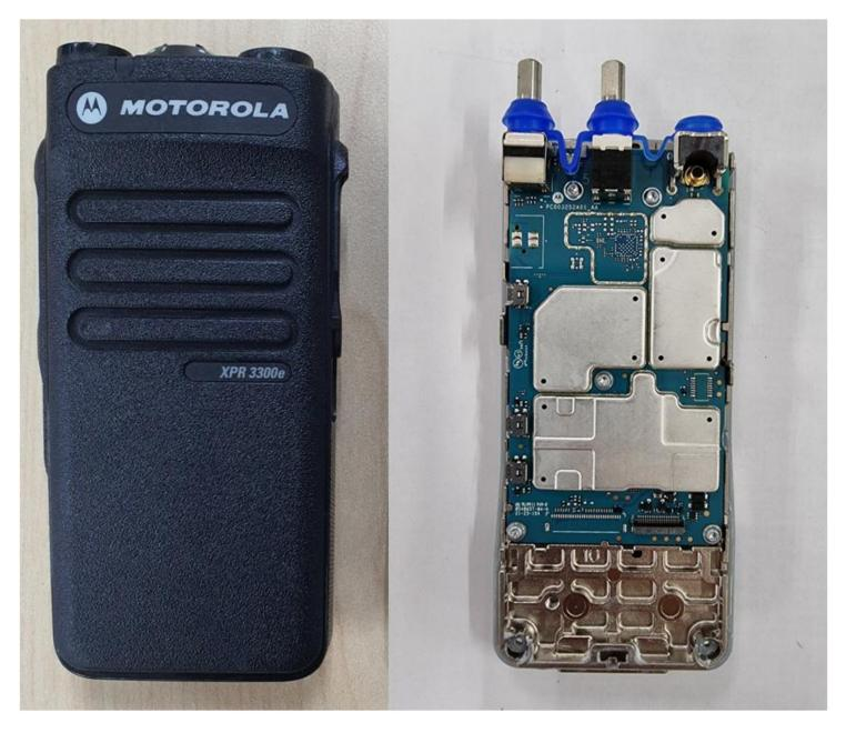
RF boards with chassis and housing for Non Keypad model (Front Side) Non-TIA4950
