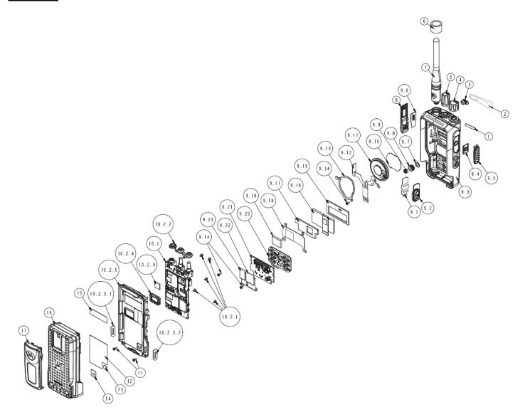
**Exploded view of Non Keypad radio**
