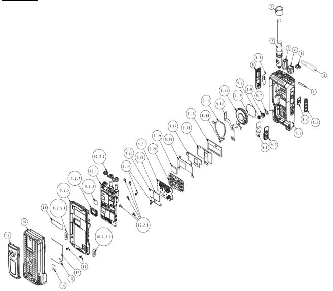
**Exploded view of Limited Keypad radio**
