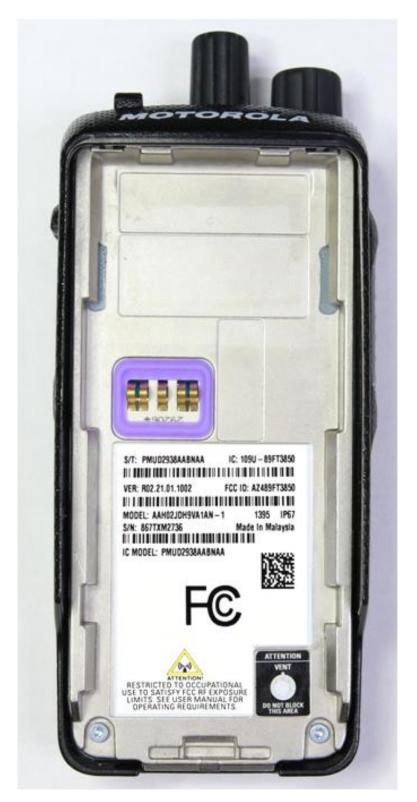
Back View for Limited Keypad and Plain Model (FCC/IC label) – XPR 3500e & XPR 3300e
