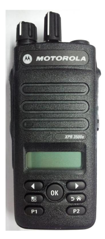
Front view with display and limited keypad model - XPR 3500e
