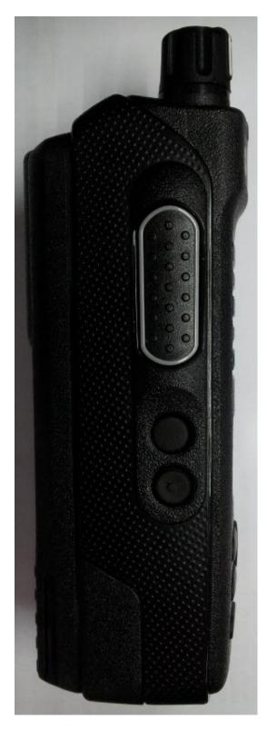
Side View for Limited Keypad and Plain Model (Left) - XPR 3500e & XPR 3300e
