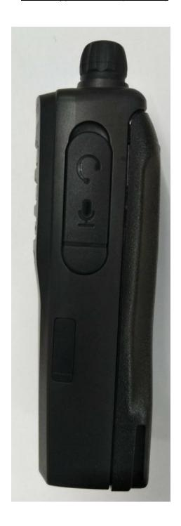
Exhibit 3E - Side view (Left) with Battery Non-Keypad model (CP200d)
