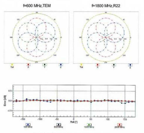
Receiving Pattern ( $\phi$ ),  $\vartheta = 0^{\circ}$
