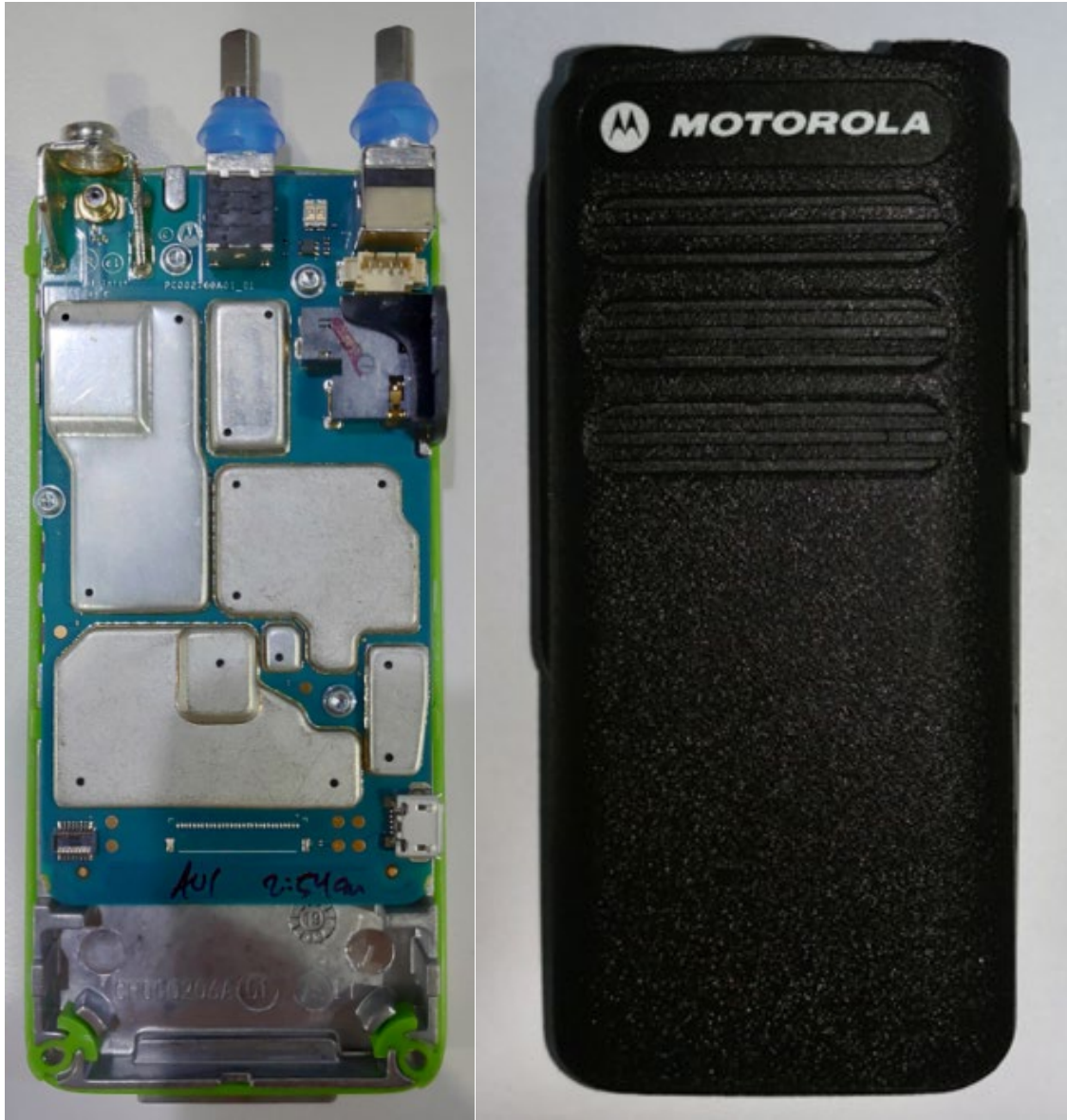
RF board with chassis and housing (front side) -Non Keypad (NKP) model, AAH87JDC9JA2AN)-
