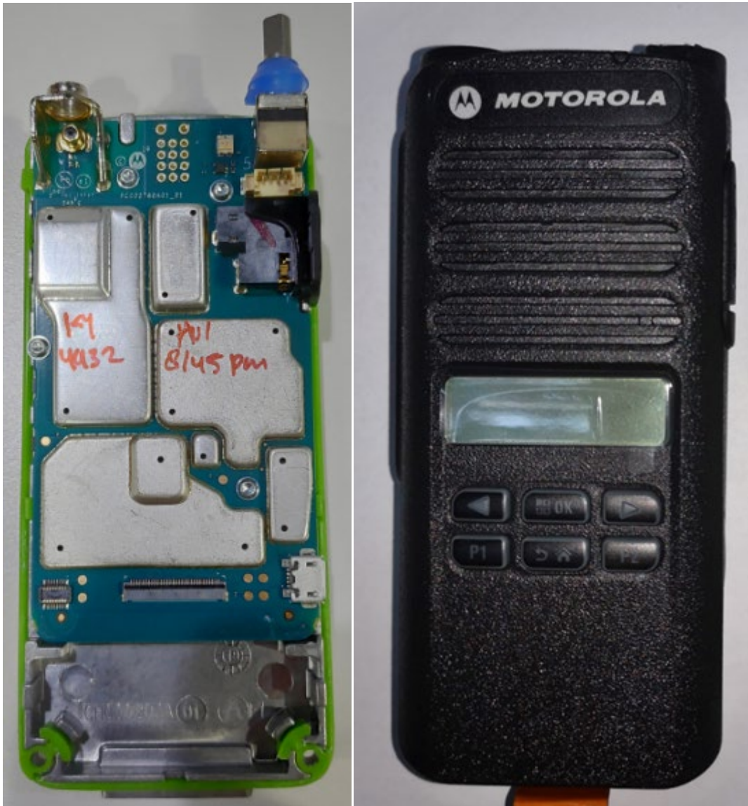
RF board with chassis and housing (front side) -Limited Keypad (LKP) model, AAH87JDH9JA2AN-
