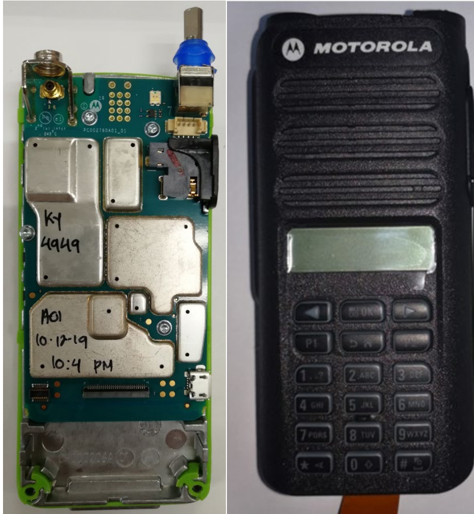
RF board with chassis and housing (front side) -Full Keypad (FKP) model, AAH87JDF9JA2AN-
