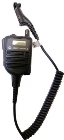
HMN4104B IMPRES Display Submersible RSM w/ jack & CH selector
