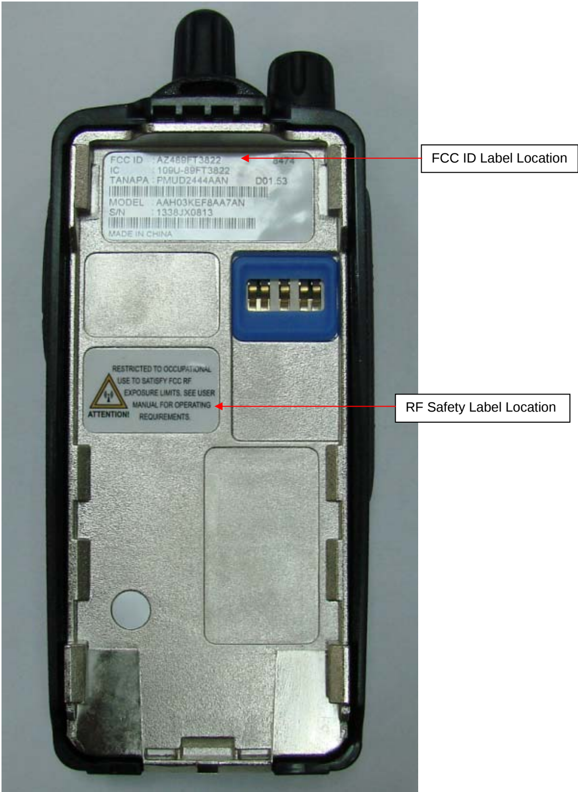
Figure 3-5: Rear view of complete radio showing FCC ID Label & RF Safety Label location
