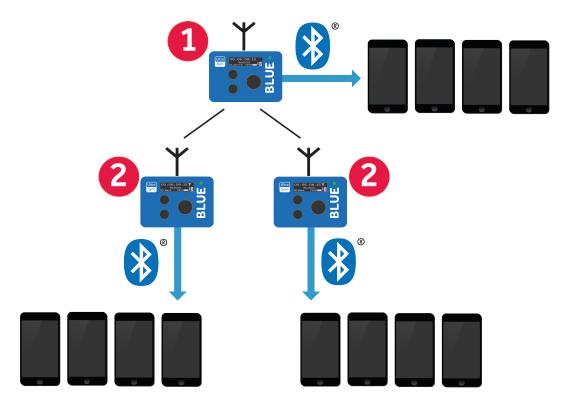
UltraSync BLUE (1) is set to run in Int Master RF TX mode and is the master in the RF network. The other UltraSync BLUEs (2) are set to run in RF Slave mode. The slaves sync with the master.
