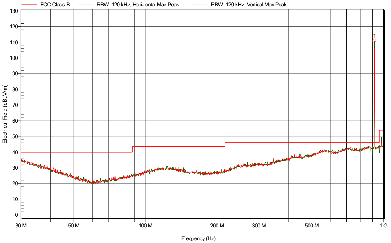
Figure 7.3.7.2 Electric field emissions Plot, 30MHz to 1GHz, Operation on 915.8MHz - Peak detector scan
