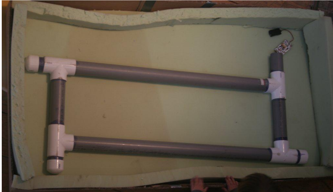
Figure 7 - Circuit board as connected to loop antenna
