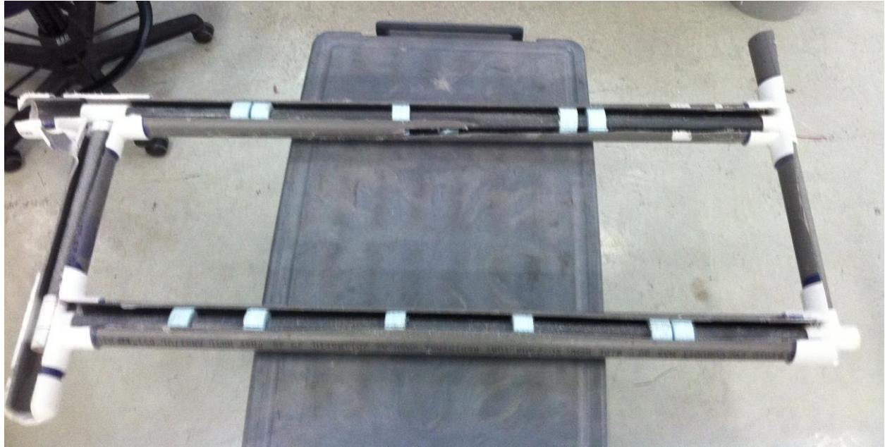
Figure 5 – Antenna - Outer PVD tubing cut to show inner PVC tubing with wire loops
