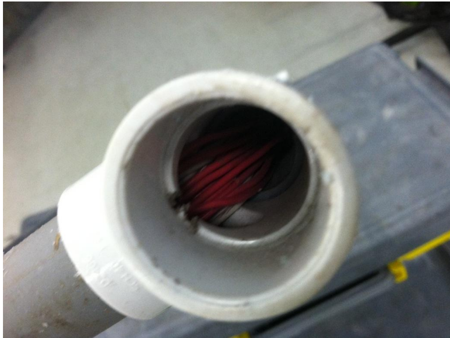
Figure 6 - Antenna winding inside inner PVC tube
