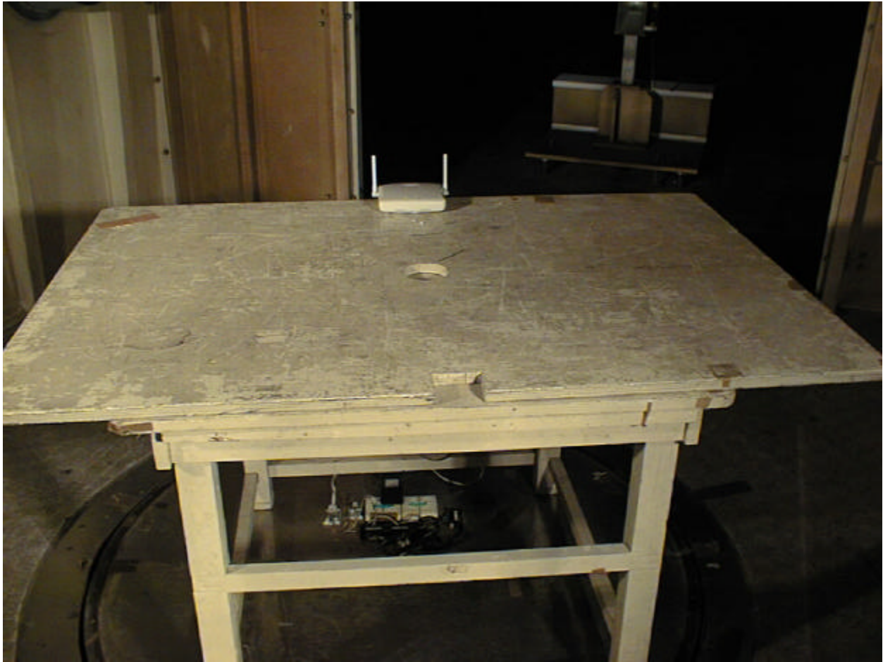
Front View of Radiated Emissions Test Set-up
