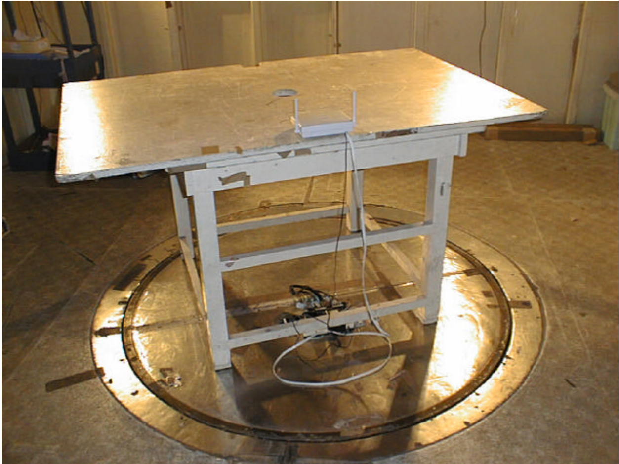
Back View of Radiated Emissions Test Set-up
