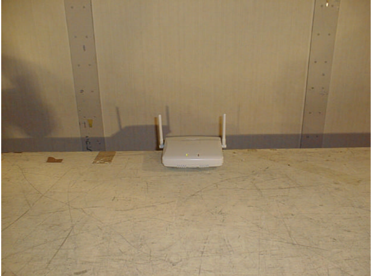
Front View of Line Conducted Emissions Test Set-up
