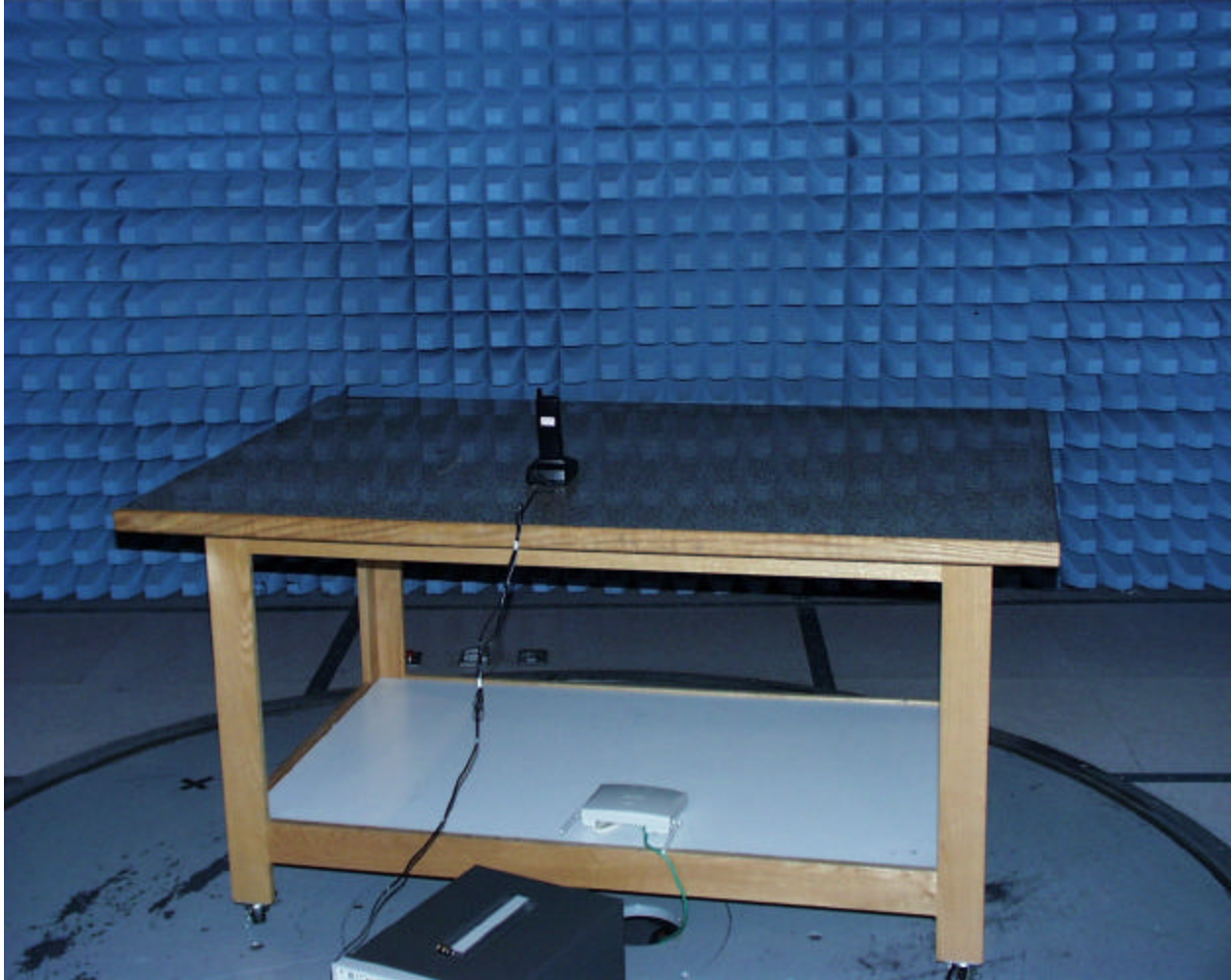
Back View of Worst Case Radiated and Line Conducted Emissions Test Set-up
