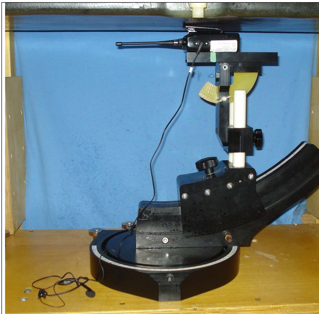
Body-worn SAR Configuration - Antenna 3, Battery a, Audio G3a
