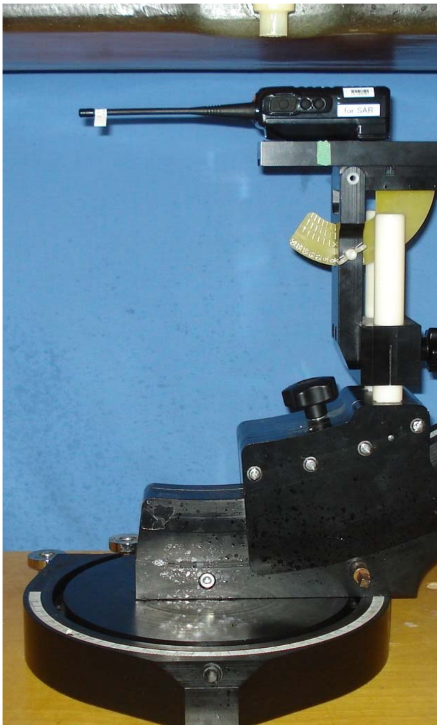
Face-held SAR Configuration Test Setup
