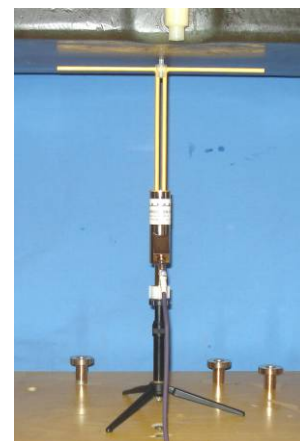
SPEAG 450 MHz Validation Dipole Setup
