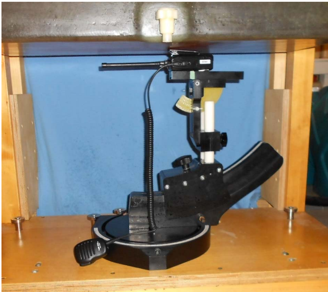
Body-worn SAR Configuration Test Setup
