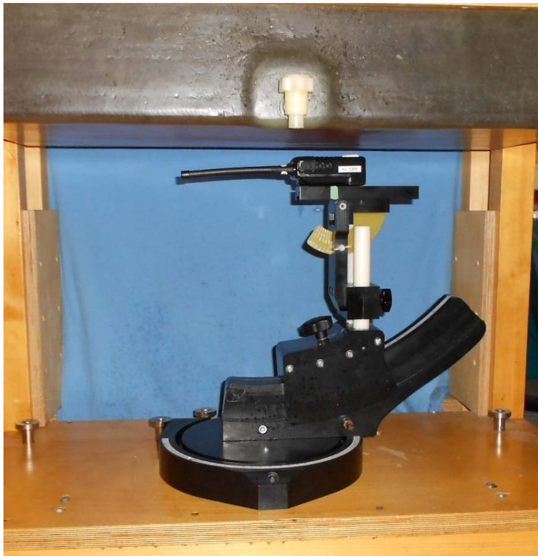
Face-held SAR Configuration Test Setup
