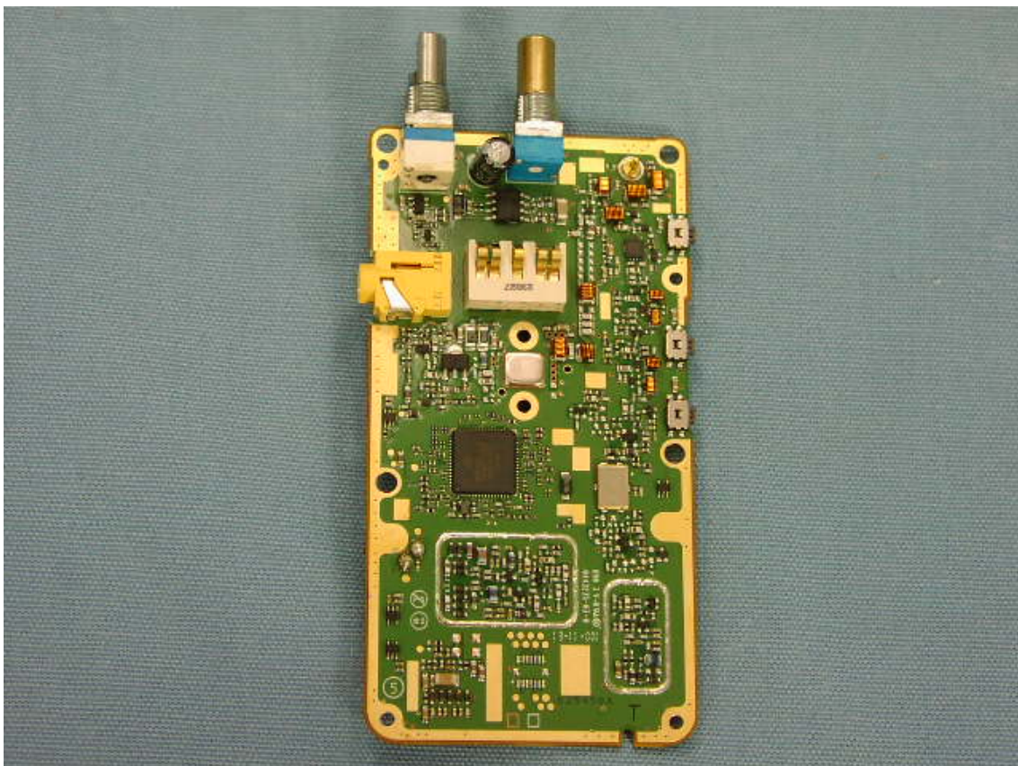
Side A of MAIN-UNIT Without VCO Case (EVX-534 / EVX-539)
