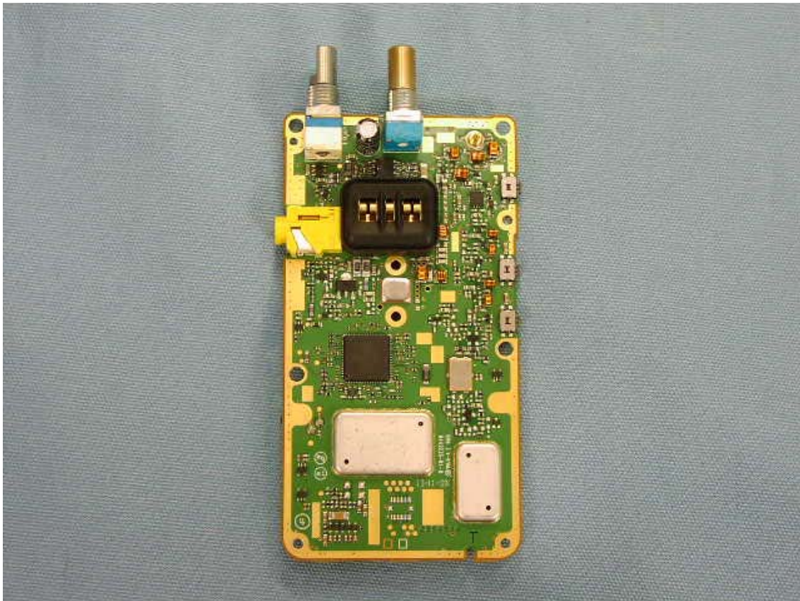
Side A of MAIN-UNIT With VCO Case (EVX-534 / EVX-539)
