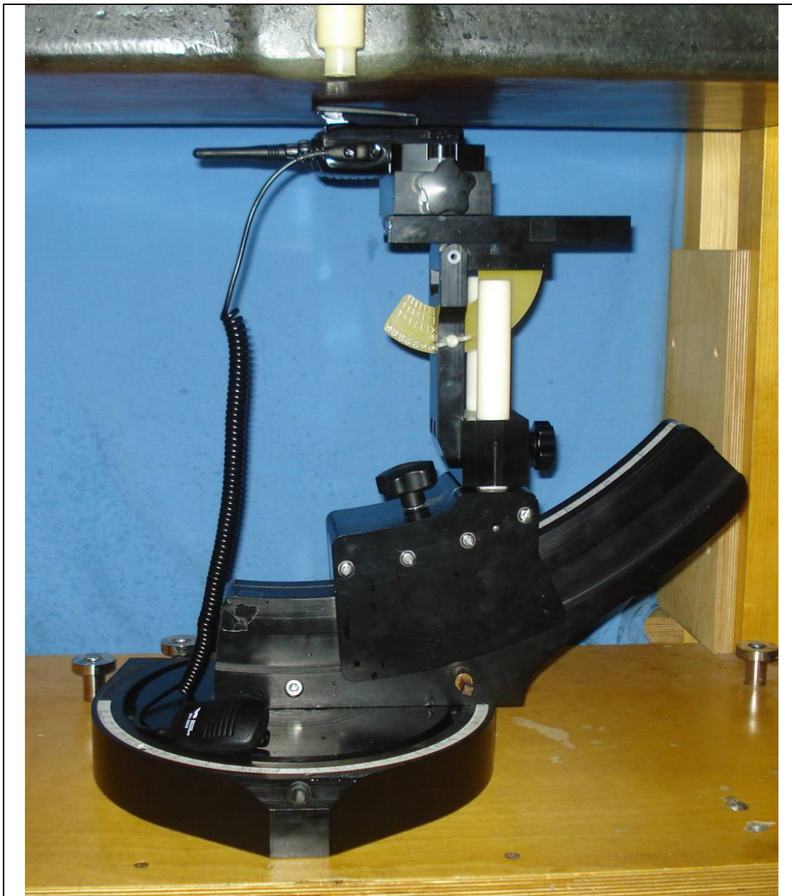
Body-worn SAR Configuration - Antenna 2, Battery a, Audio G1a
