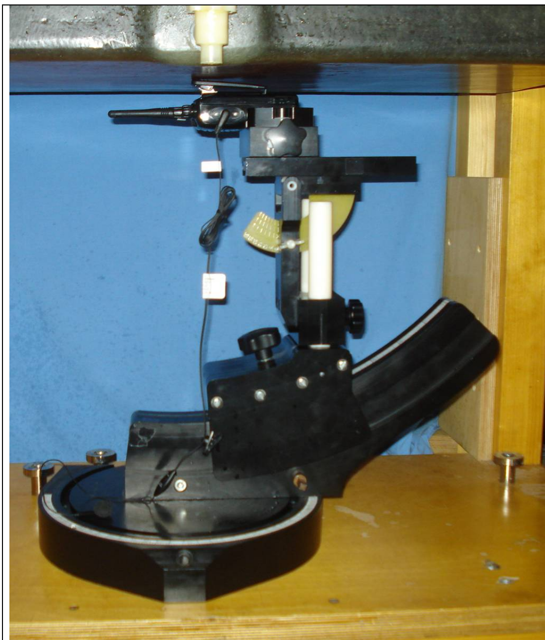
Body-worn SAR Configuration - Antenna 2, Battery a, Audio G3a
