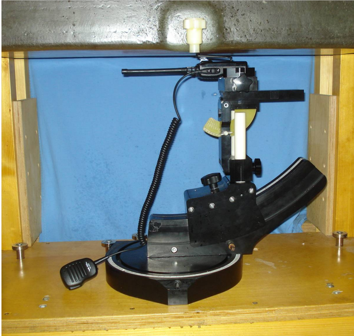
Body-worn SAR Configuration Test Setup
