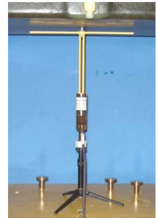
SPEAG 450 MHz Validation Dipole Setup
