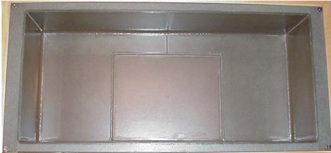
Fiberglass Planar Phantom - Top View
