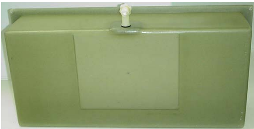
Fiberglass Planar Phantom - Bottom View
