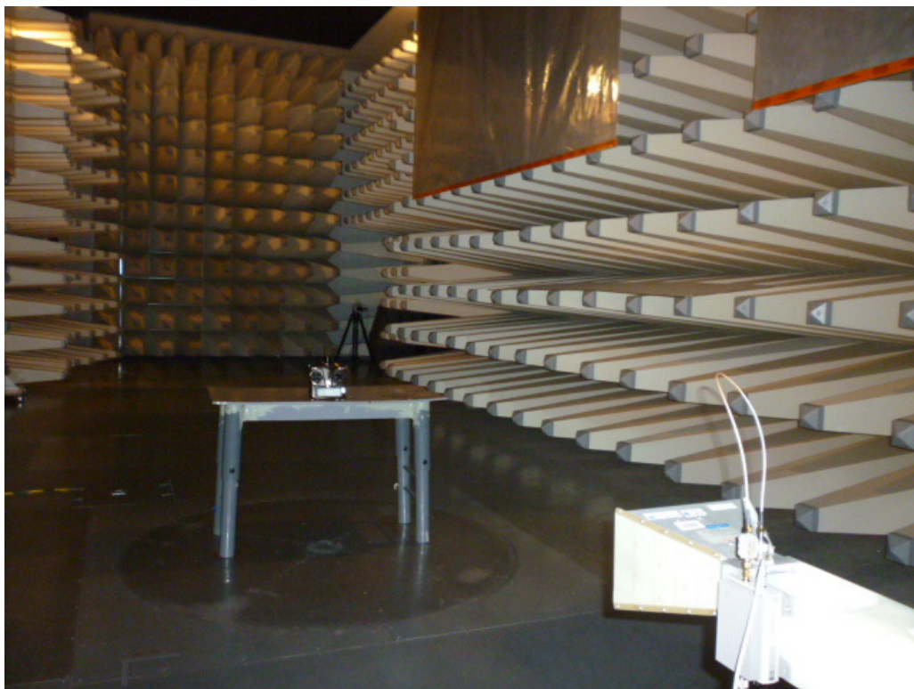
Set-up for Radiated Emission (Transceiver)
