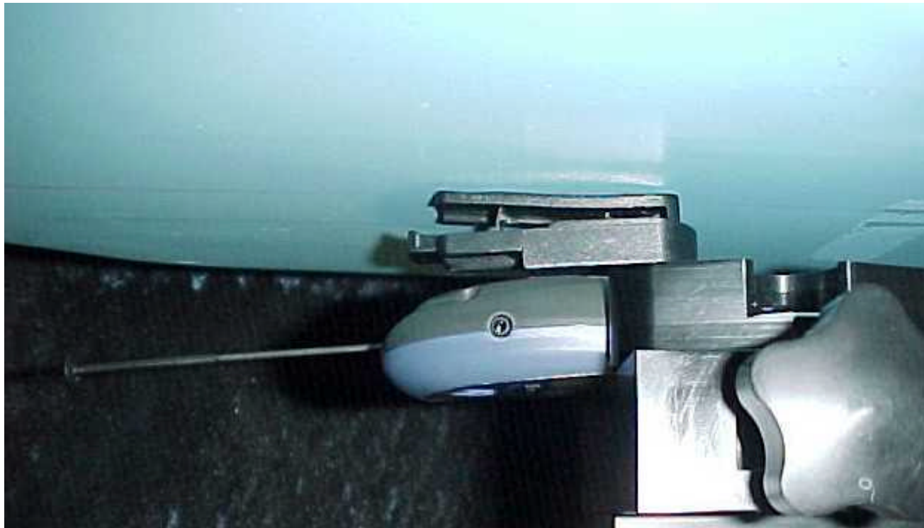
Position of device against flat phantom using carry accessory SXX 107 6820/55.
