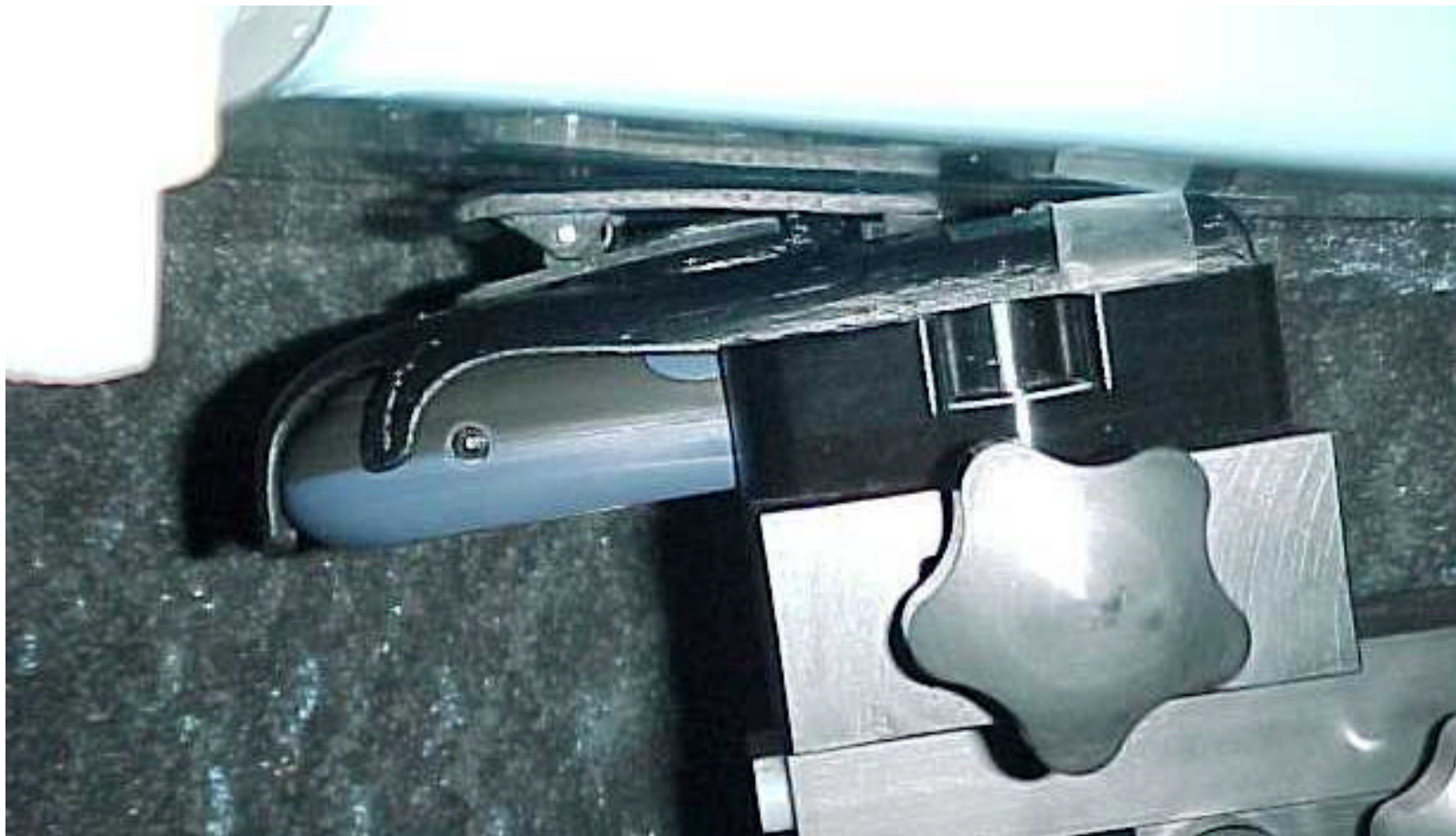
Position of device against flat phantom using carry accessory SXK 109 4705. Back of the phone against the holster
