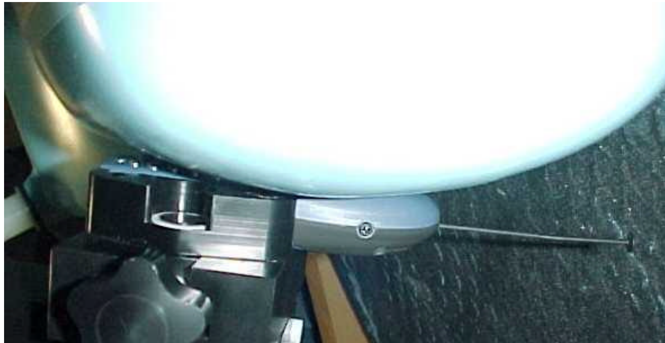
Position of device against head phantom with the antenna extended
