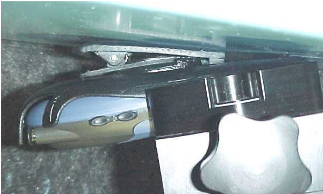
Position of device against flat phantom using carry accessory SXX –109-4705. Front of the phone against the holster.
