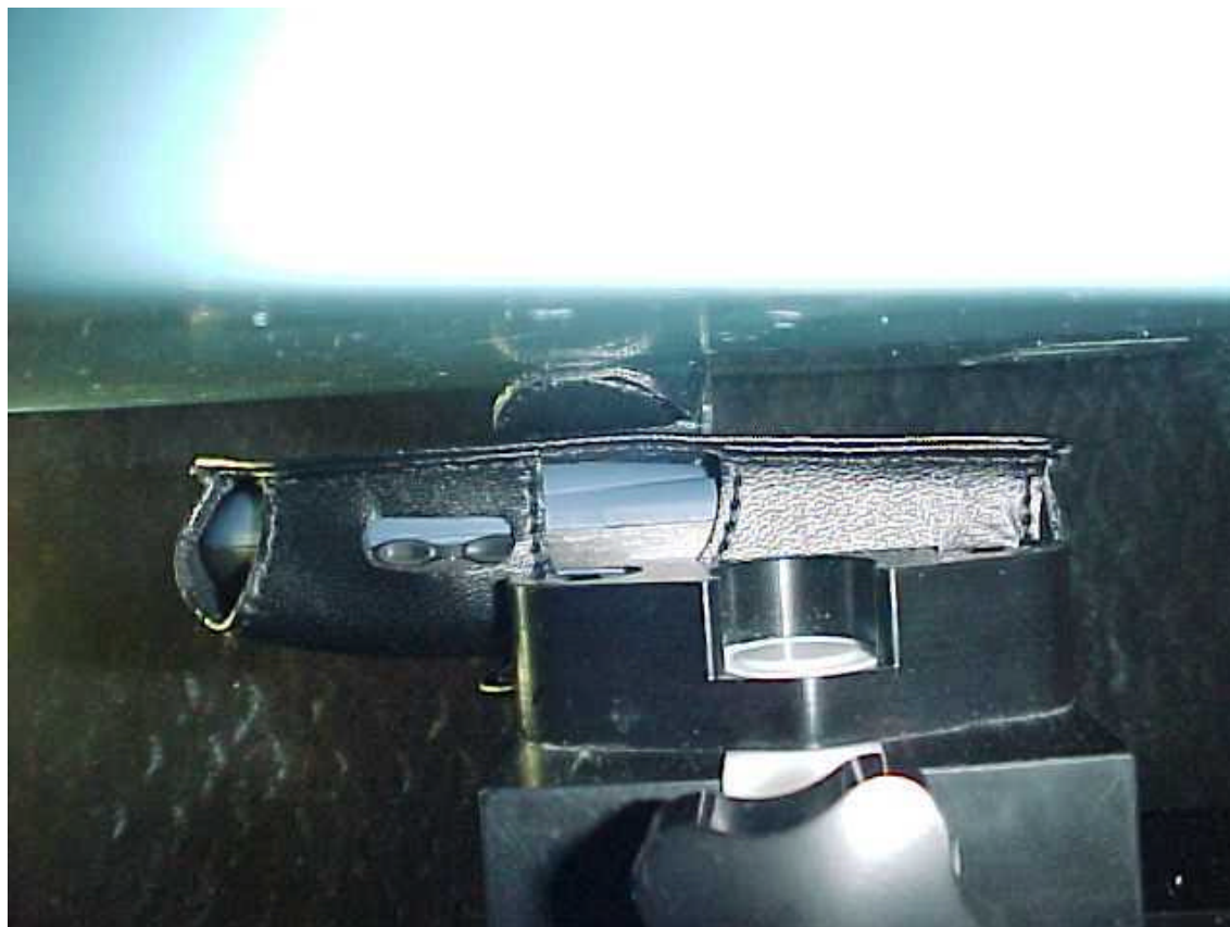
Position of device against flat phantom using carry accessory SXX -109-4518/1
