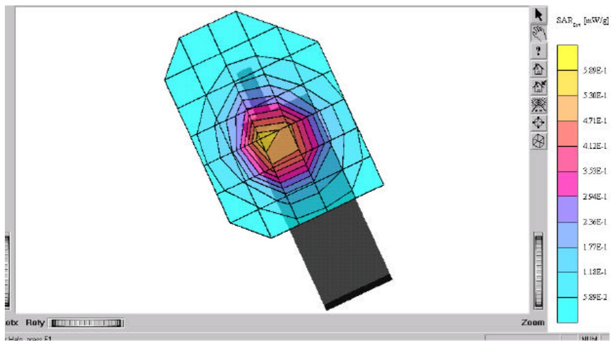
SAR distribution plot for I888 WORLD in PCS 1900 mode on f=1850.2MHz and P=30.6dBm.
