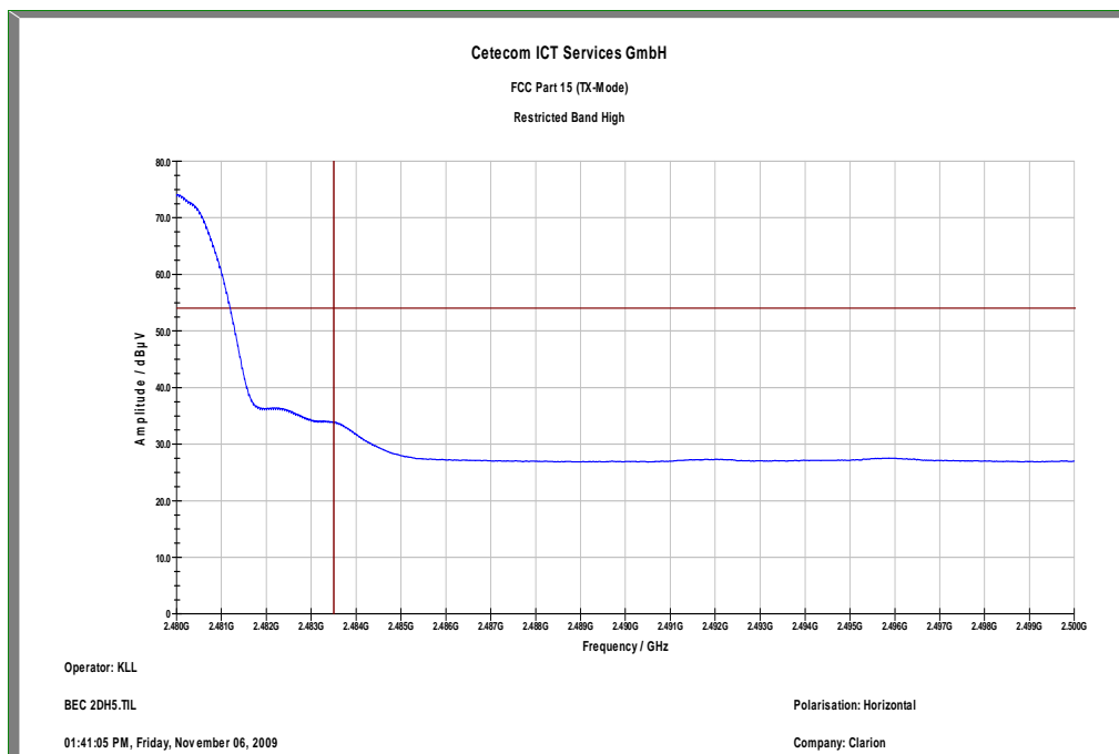
Plot 2: Restricted Bands high, DUT worst case position, vertical antenna polarization
