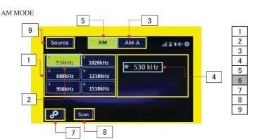
Preset Channel List Preset Channel Key Band Display Area Frequency Display Area Band Select Key STEREO Display Area Setting Key
