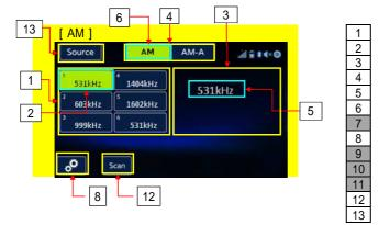
Preset Channel List Preset Channel Key Receiving Station Display Area Band Display Area Frequency Display Area Band Select Key STEREO Display Setting Key TA Icon Display Area NEWS Icon Display A: Radio Text Display Area SCAN Key Source Select Key
