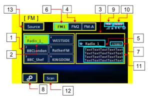
Preset Channel Key Receiving Status Display Area Band Display Area Frequency Display Area Band Select Key STEREO Display Area Setting Key TA Icon Display Area NEWS Icon Display Area Radio Text Display Area SCAN Key Source Select Key
