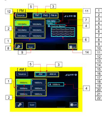
Preset Channel List Preset Channel Key Band Display Area PS Name or Frequency Display Area Band Key Radio Text Display Area STEREO Display Area Setting Key SCAN Key Tag Key Frequency Display Area Source select Key Bookmark Key List Key **HD** Indicator Live Indicator Receiving MultiCast Display Area MultiCast Select Key Short Name Display Area Artist Experience Display Area Song Name Display Area Artist Name DisplayArea
