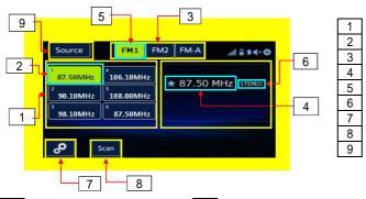
Preset Channel List Preset Channel Key Band Display Area Frequency Display Area Band Select Key STEREO Display Area Setting Key SCAN Key Source Select Key
