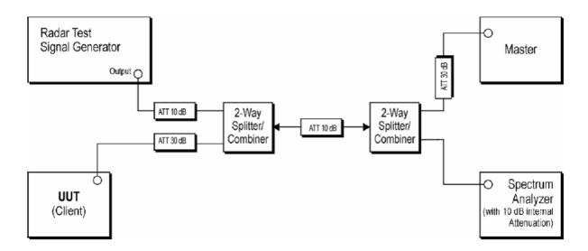
A-50-ohm load is connected in place of the spectrum analyzer, and the spectrum analyzer is iconnected to a coaxial cable. The radar signal generation equipment consists of a vector signal generator
