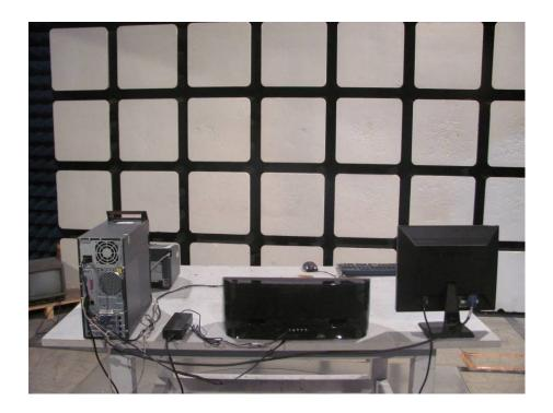
AC Power Conducted Emission Test
