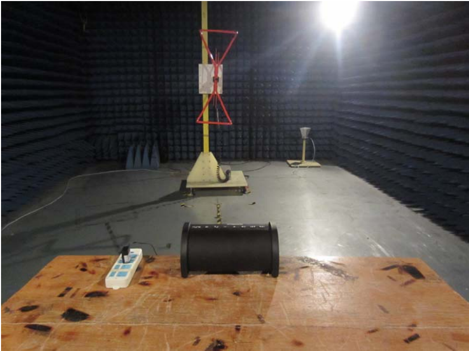
RE TEST SETUP
