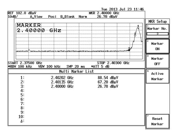
According to the page 13 of this report, the emission of the fundamental frequency 2402.0MHz is 89.3dBuV/m and 88.0dBuV/m for peak and average level respectively. Based on the delta method, the emission at the bandedge, 2400MHz, is more than 50dB below the fundamental and 20dB bandwidth falls in assigned band. It is deemed to comply with section 15.215. Besides, it is below the limit of 74dBuV/m and 54dBuV/m for peak and average level under 15.209. It is deemed to comply with section 15.249(d).
