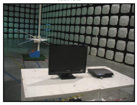
Above 1GHz: (full anechoic chamber)
