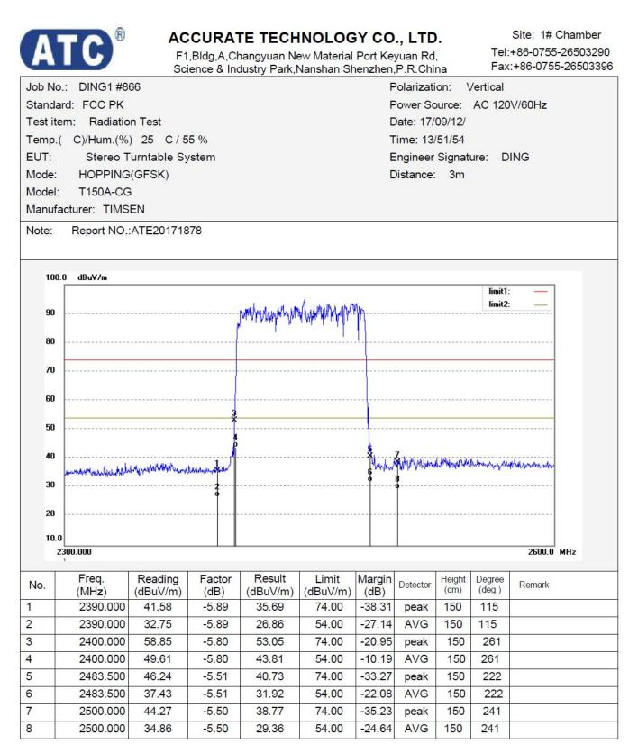
Note: Average measurement with peak detection at No.2&4&6&8
