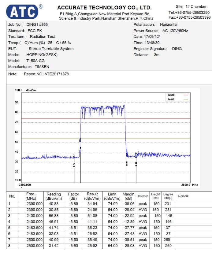
Note: Average measurement with peak detection at No.2&4&6&8
