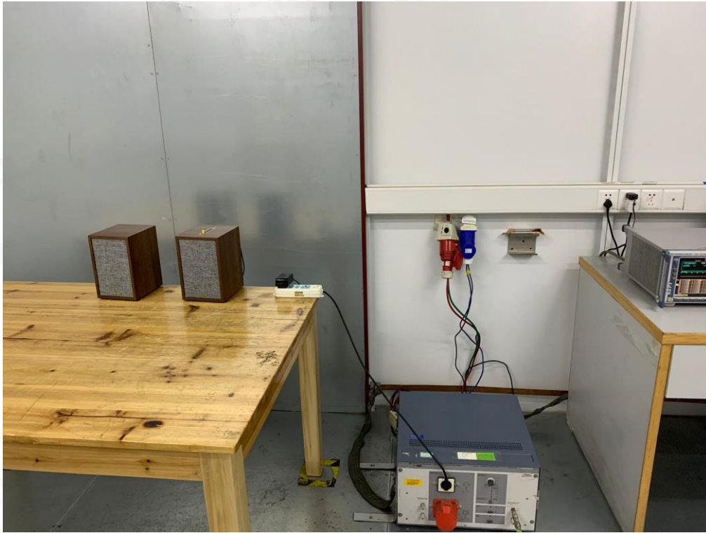
CONDUCTED TEST SETUP
