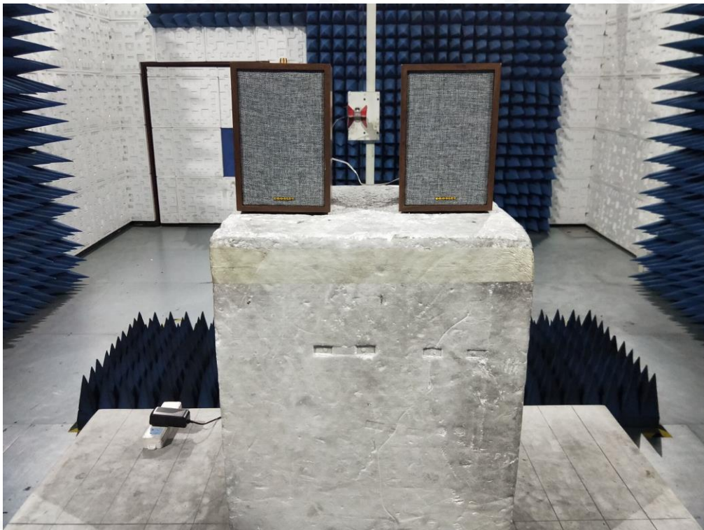
RADIATED EMISSION TEST SETUP ABOVE 1GHZ
