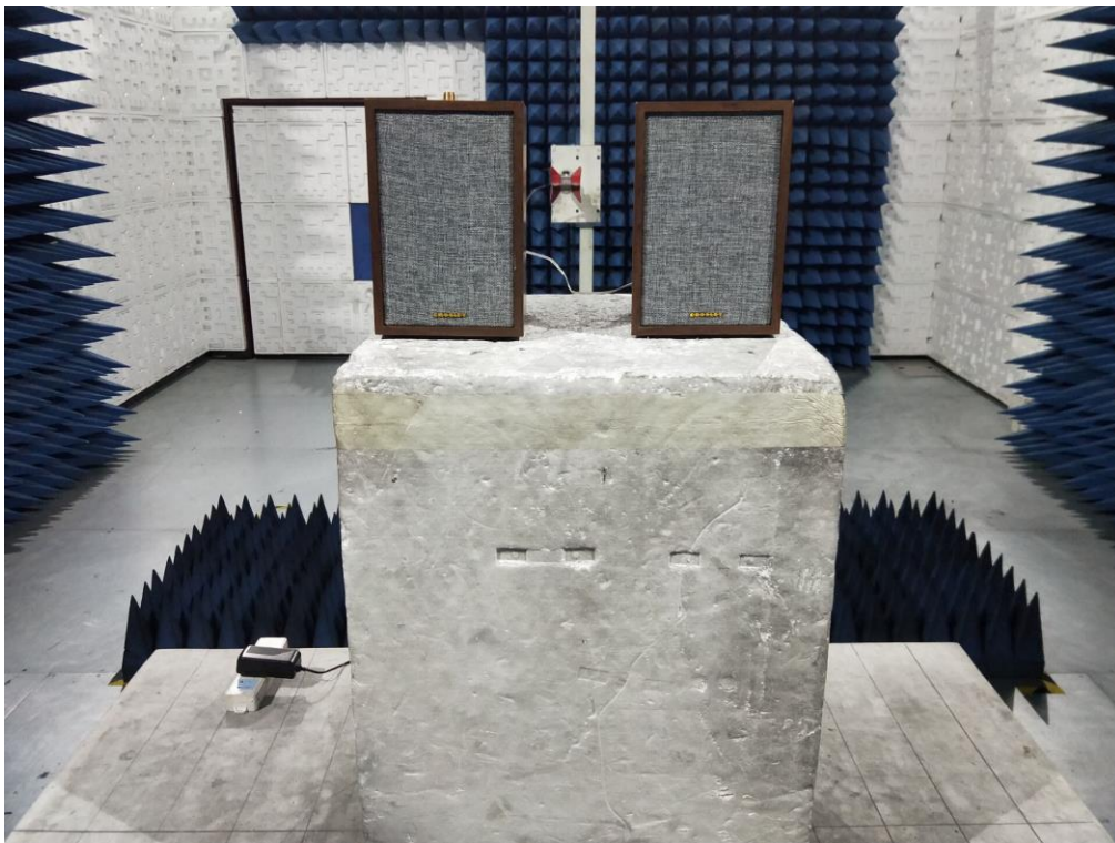
RADIATED EMISSION TEST SETUP ABOVE 1GHZ
