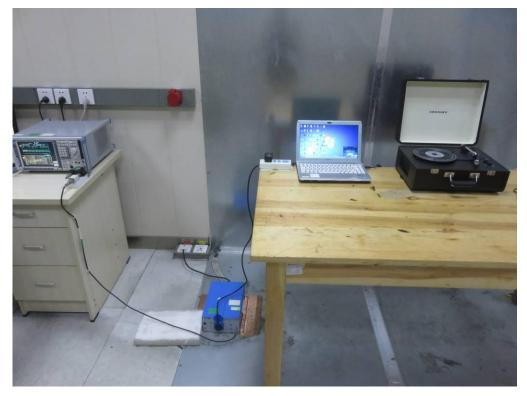
FCC RADIATED EMISSION TEST SETUP
