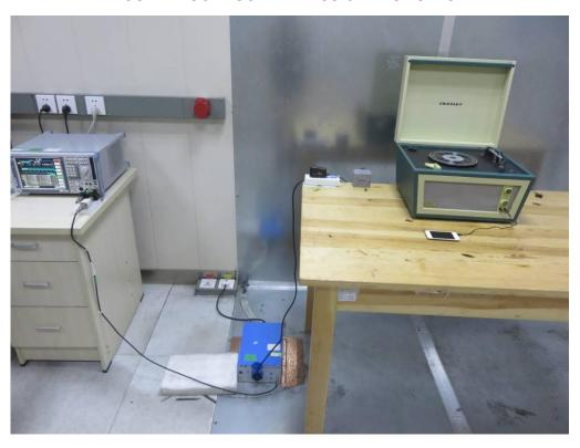
FCC RADIATED EMISSION TEST SETUP
