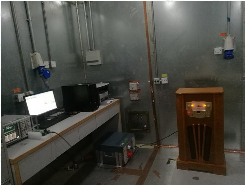
FCC RADIATED EMISSION TEST SETUP
