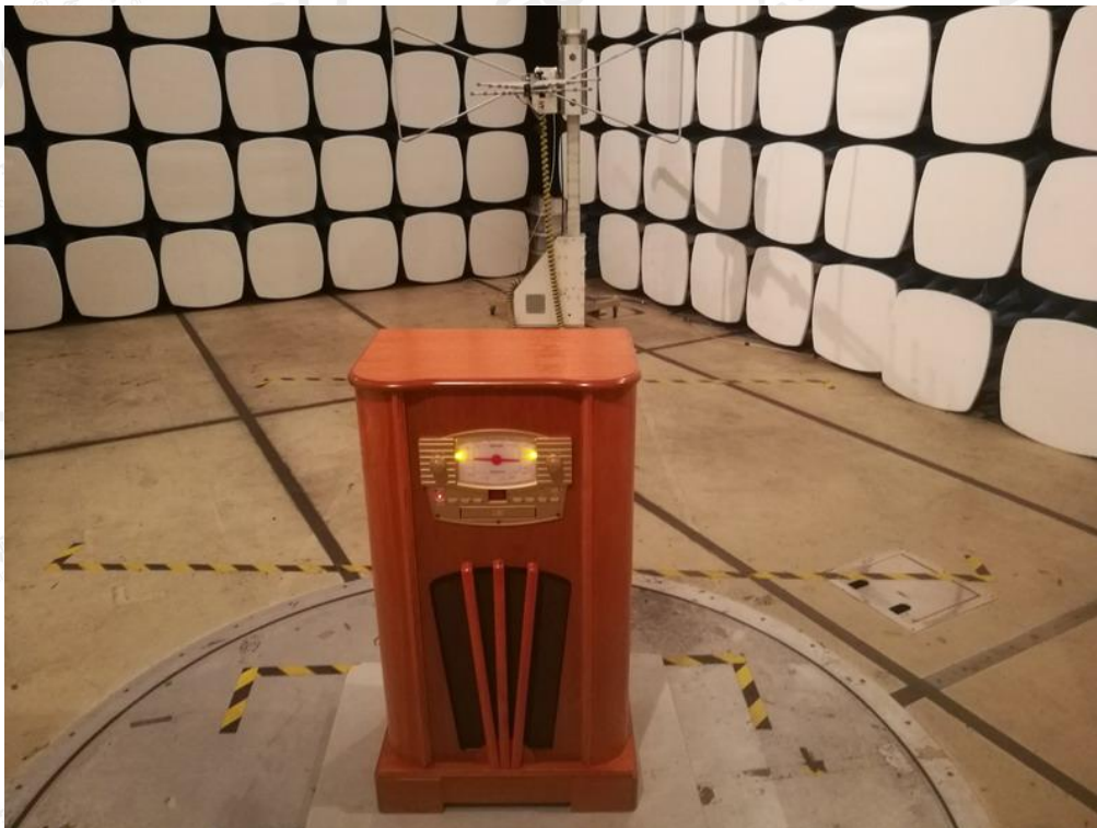
FCC RADIATED EMISSION TEST SETUP
