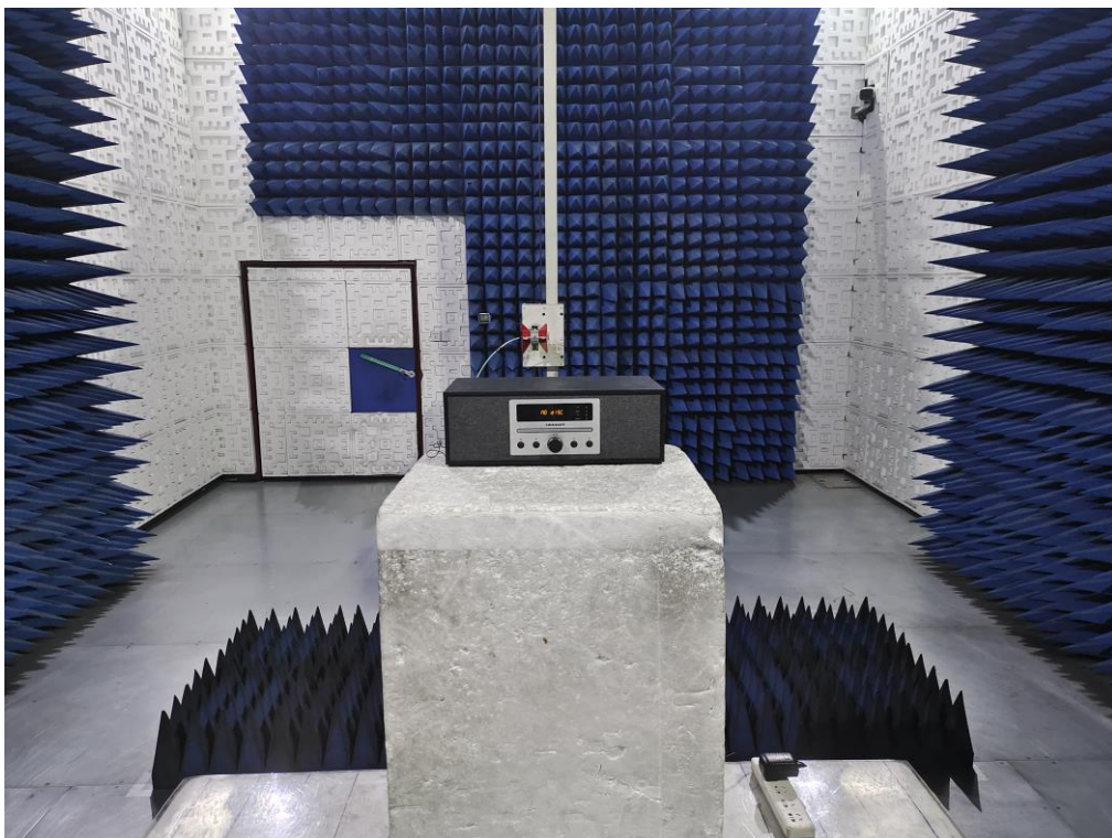
RADIATED EMISSION TEST SETUP ABOVE 1GHz
