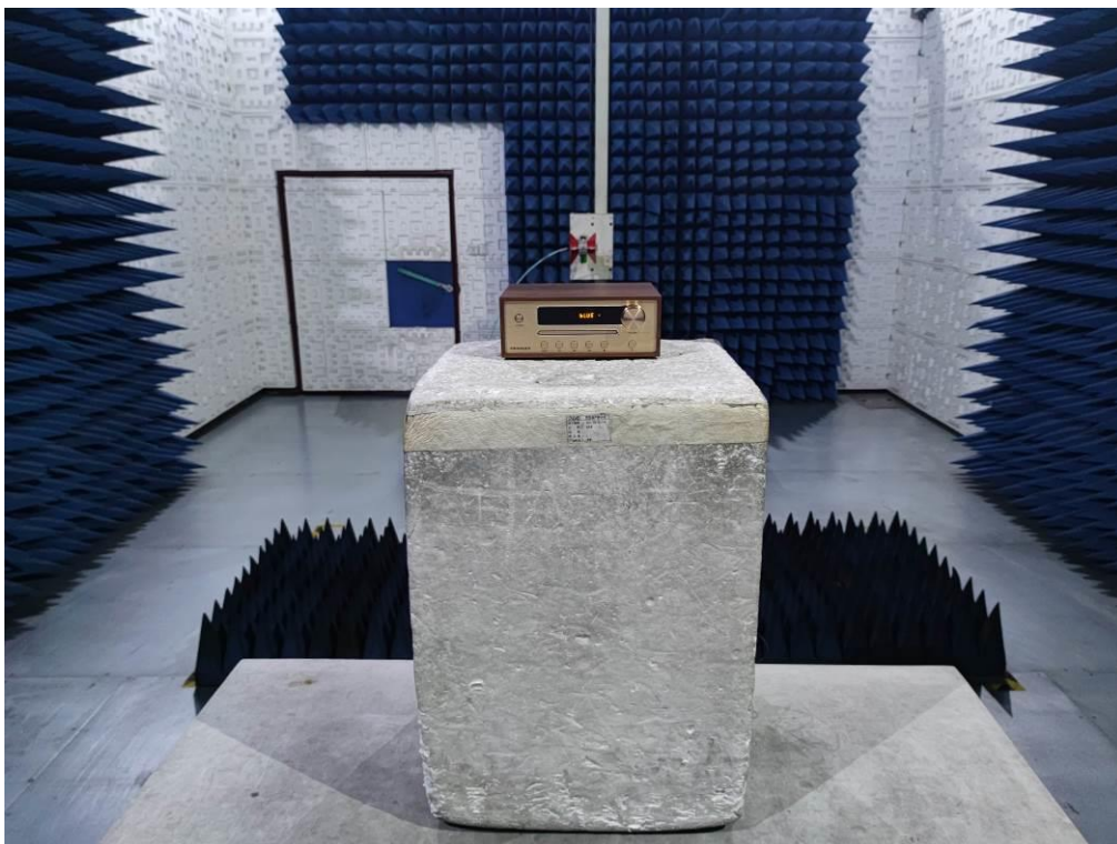
RADIATED EMISSION TEST SETUP ABOVE 1GHz
