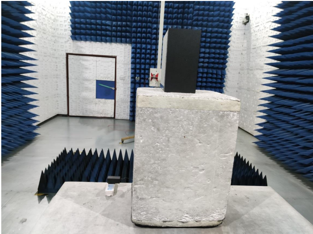
RADIATED EMISSION TEST SETUP ABOVE 1GHz
