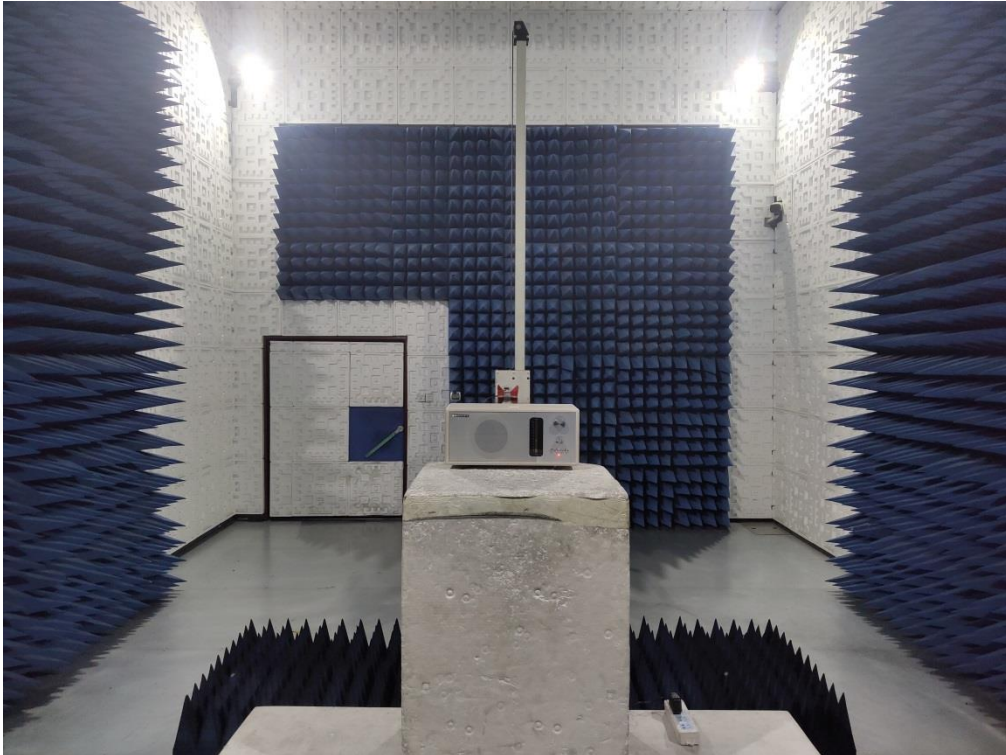
RADIATED EMISSION TEST SETUP ABOVE 1GHZ
