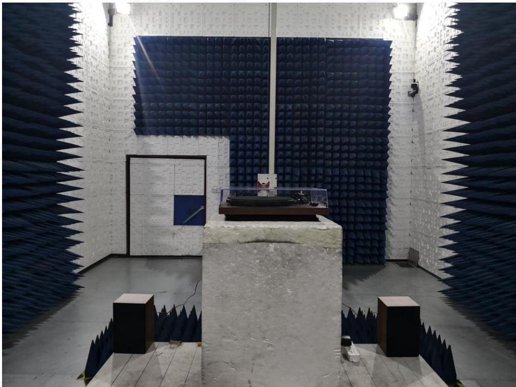
RADIATED EMISSION TEST SETUP ABOVE 1GHZ
