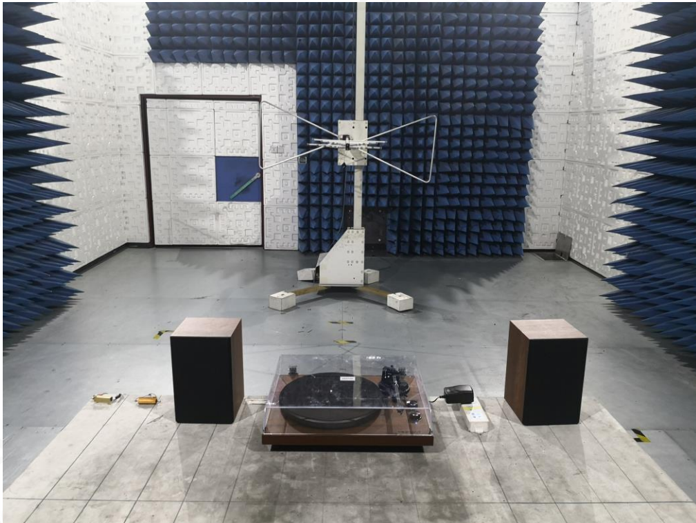
RADIATED EMISSION TEST SETUP ABOVE 1GHZ
